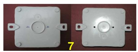
Picture 7: Mark and drill two holes on the bottom of the box for the contact screws (3mm holes). The distance between the two holes depends o the distance of the holes in the radiator rods (you should have remembered this). These holes are used for the 3,9 x 16 mm
