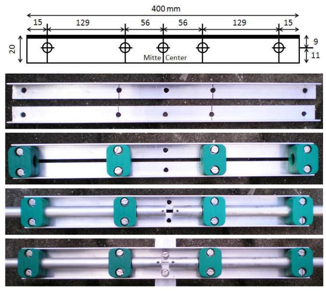
The break of the radiator rod in the middle has to be 10-15 millimetres. This distance has to be cut from the length of the middle 16mm rod, because the middle rod has to be exactly 2,00m from tip to tip, including the spacing in the middle. Drill 3,5mm holes into the inner ends of the rod, you need them for the contact screws. Remember the distance between the two holes, you will need them for the connection box.
