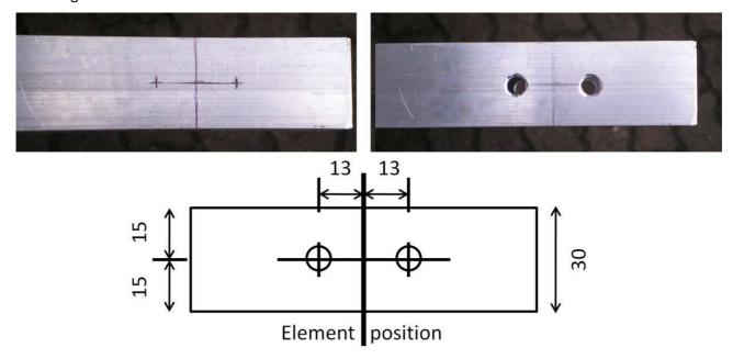
Template for the drills on the aluminium bar:
