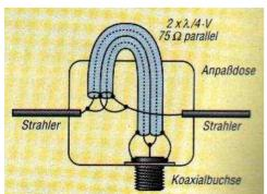
The choke needs a length of lambda/4 multiplied with the shortening factor "V" of the cable. Only the fully shielded length of the cable counts to the total length, soldering lugs do not count to the length and should be as short as possible. It could make problems if the solder lugs on the radiator side are too long, because they would "stretch" the dipole some millimetres and you could get mismatching in the system.
