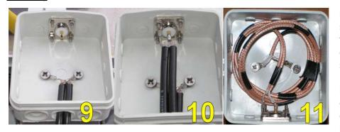
Picture 9: On the one end solder the 4mm cable shoes to the ends and connect the choke with the 3.9 x 16 mm screws to the radiator tubes. If you are using RG59 you have to carry the choke outside of the box, make a coil outside the box and lead it back into the box. Picture
