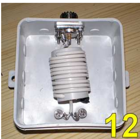
Picture 12: In fact this isn't really a choke, it's only a coil for suppression of the sheath current. 50 Ohm systems do not need a transformation. The choke has about 10 windings of thin coax cable on a 25 mm diameter PVC tube. The number of windings is uncritical, but it should have at least 7 windings for good suppression. Solder one end to the coax socket - connect the outer conductor with a 3mm cable shoe to the M3x12 screw. Solder the other end to the two 4mm cable shoes and fix them with the 3.9 x 16 mm contact screws to the radiator tubes. Now your antenna should be ready.
