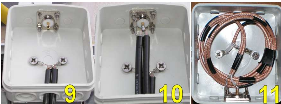
Picture 10: In the inner it will be soldered to the coax socket. The inner conductors to the inner contact and the outer conductors to a 3mm cable shoe, which will be connected to one M3x12 screw at the coax socket. Picture 11: If you are using RG179 or RG188 PTFE cable, you can wind it to a coil and leave it completely in the box as shown in the picture.
