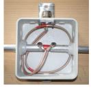
RG59 and RG179, will fit into the box. With RG59 it could be a bit tricky, so you maybe have to try first with a better position for the radiator, because RG59 is relatively stiff.
