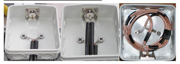
Now connect the one end to the dipole rods with the 4mm cable shoes and the self-tapping screws BS3.9x16. The other end will be connected to the coax socket. Solder the inner conductor to the middle contact, the shield with the 3mm cable shoe to one of the 3mm screws which hold the coax socket - this is the ground.
