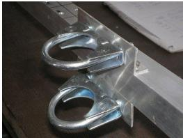
Find the balance point of the antenna first and make a marker on or near this point. There should be the middle of the mast clamp brackets too.
