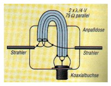
The DK7ZB match matches the 28 or 12.5 ohm impedance of the dipole to 50 ohms you need for connecting your transceiver and feeding cable. The picture shows you the schematic of this match.
