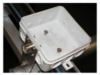
Then you can mount the box on the dipole. Make the holes through the bottom of the box for the contact screws (distance of the holes is 20mm). Do not make the holes too big. For testing you may attach the screws now, but don't screw them to hard in now.
