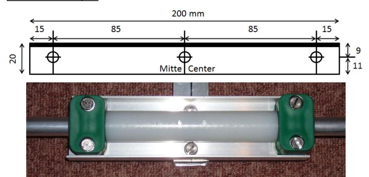
The dipole holder consists of two pieces of angled aluminium (20x20x2mm) with each 200mm length, which are mounted across the boom. 25mm plastic pipe clamps are attached at the ends. They are fastened with Z6x45mm screws (don't forget the flat washers!) to the aluminium brackets. The aluminium brackets are also mounted with Z6x45mm screws to the boom. The dipole connector will be clamped between the pipe clamps.
