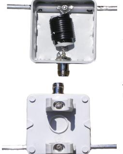
Cut the lugs from the end of the box. On the one side cut a 16mm hole into the membrane for the coax socket. For mounting the box on the boom you need two holes through the bottom. One at the dipole position, and the other at the opposite side (please check that the screw and the coax socket are not short-circuited). In our sample the hole for the dipole was about 8mm away from the wall, and on the coax side it was 16mm away from the wall (here you need more space because of the coax socket.
