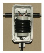
**Attention:** The picture shown left shows a connection box for the lightweight construction. For our aluminium version a bigger 85x85mm box is being used. The small box should be used for the connection box!
