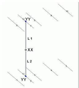
Two yagis with 25 Ohm impedance can be stacked easily. You need two pieces of 50 Ohm coax cable with an odd-numbered multiple of  $\lambda/4$  length (e.g.  $3\lambda/4$ ,  $5\lambda/4$  and so on) considering the velocity factor of the cable type (e.g. 0,67 for RG58 or 0,82 for Aircell 5). For practical usage a length of  $5\lambda/4$  is perfect. It's also possible to use  $7\lambda/4$  or longer, but you will have more cable losses.
